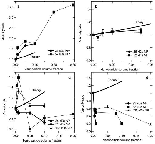
Figure 10. Viscosity ratio of the nanoparticle blends with respect to pure polystyrene as a function of nanoparticle volume fraction, with different molecular weight linear polystyrenes' at 170°C: (a) 19.3, (b) 31.6, (c) 75, and (d) 393 kDa. The curves labeled theory are the values predicted by Batchelor's relation for this system, ending at the limit of the relation's applicability  $(\phi \sim 0.1).$
