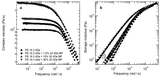
**Figure 7.** Complex viscosity (a) and storage modulus (b) data for pure PS 19.3 kDa and its blends with 52 kDa NP at 170 °C. Both these properties increase at all frequencies upon nanoparticle addition. Same symbols used in each graph.
