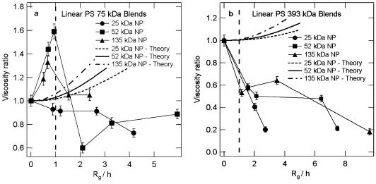
Figure 4. Viscosity ratio of the nanoparticle blends with respect to pure polystyrene for two different entangled systems, PS 75 kDa (a) and PS 393 kDa (b) at 170 °C. The curves labeled theory are the values predicted by Batchelor's relation and these end at the limit of the relation's applicability ( $\phi \sim 0.1$ ). The viscosity falls precipitously when the radius of gyration is greater than the interparticle half-gap for the entangled systems.
