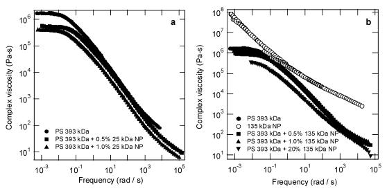
**Figure 6.** (a). Complex viscosity as a function of frequency for pure PS 393 kDa and its blends with 25 kDa NP at 170 °C. In this case, the viscosity is decreased at all frequencies. A large viscosity reduction is apparent with just 1% addition of the nanoparticles. (b) Complex viscosity as a function of frequency for the blends of 135 kDa NP with PS 393 kDa also at 170 °C. Here, only the terminal viscosity is reduced with nanoparticle addition until the concentration reaches 20%.
