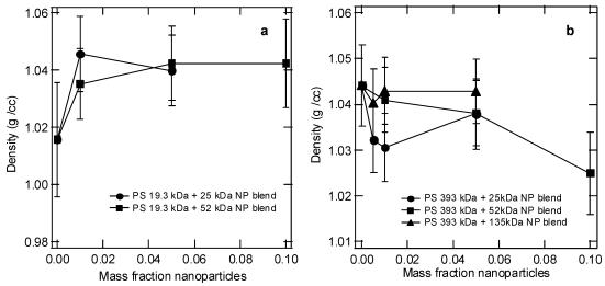
**Figure 8.** Bulk density variation as a function of nanoparticle concentration for PS 19.3 kDa blends (a) and PS 393 kDa blends (b) at 25 °C. For polymer molecular below  $M_c$ , the density increases, and when it is above  $M_c$ , the density decreases or remains constant, on nanoparticle addition.
