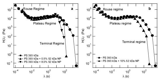
**Figure 9.** Relaxation spectra for pure PS 393 kDa and its blends with 52 kDa NP up to concentrations of 8% (a) and for a concentration of 10% (b). The Rouse, plateau, and terminal regimes are also shown. It can be seen that the nanoparticles only affect the terminal regime, by reducing the longest relaxation time, at lower concentrations while at higher concentrations, a reduction occurs at all relaxation times.
